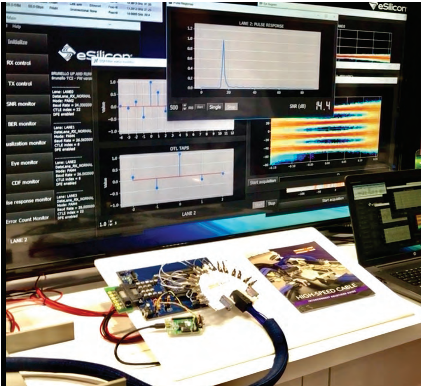
Figure 4. Real-time SerDes test data display
